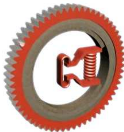
Fig 5.1 FRICTION CLUTCH WITH MAIN GEAR
