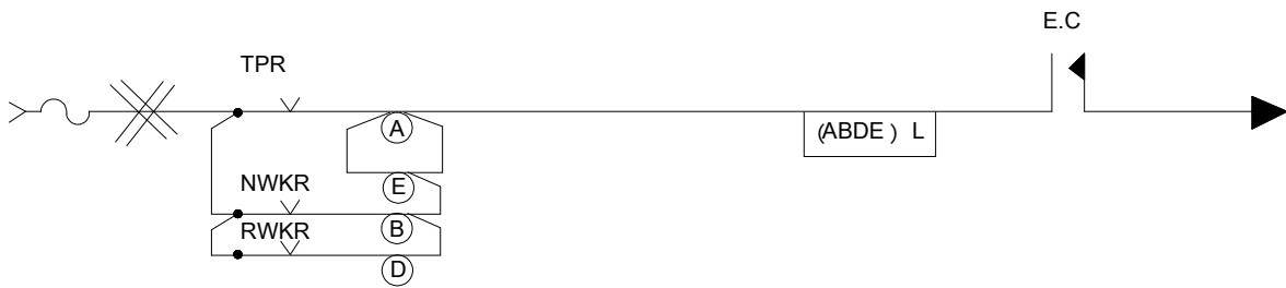
Fig. 1.5 COMBINED CIRCUIT OF TRACK AND INDICATION LOCKING
