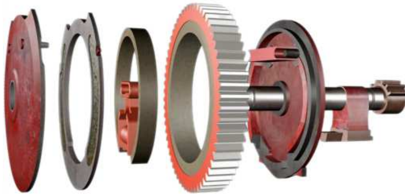
Fig : 4.3 TRANSMISSION SHAFT WITH FRICTION CLUTCH, LOCKING SEGMENT & PINION
